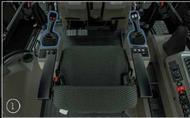
1 Shifter Button for Backhoe or Loader Function
