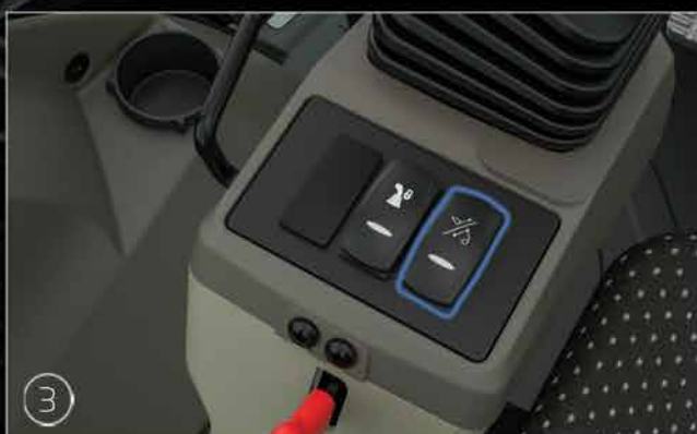
3 Shifter Button for Backhoe or Loader Function
