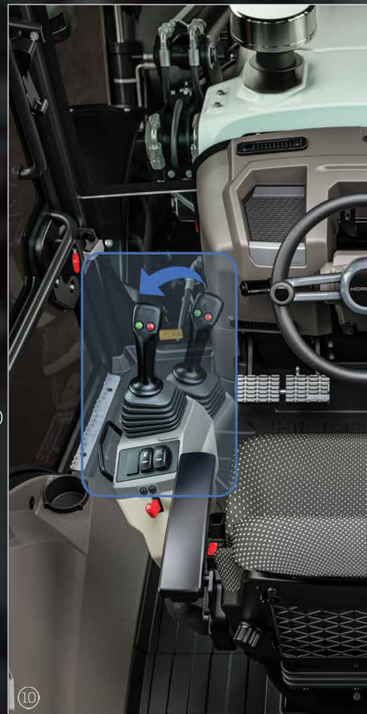
10 Tilting of the left joystick to some extent for the operator to work more comfortably on the loader side
