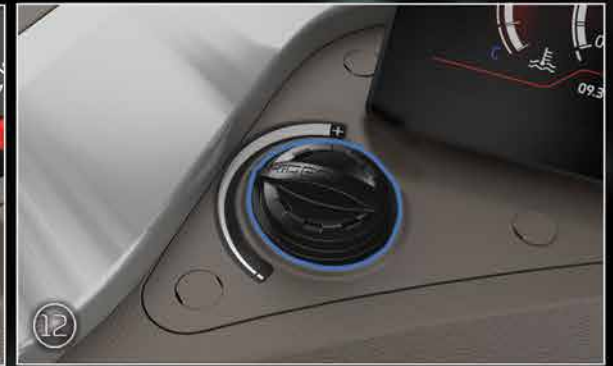
Hand Throttle with Electronic Rotary Control (*)
