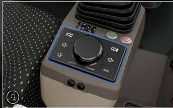
9 Opera Control Button Integrated in the Seat (**)
