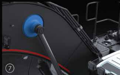
Reinforced boom cylinder cast bearing
